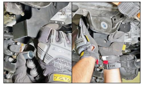
Install the 14mm bolts thru the factory axle bracket hole, the new bracket and the steel sleeve. This may require a little tap to get everything aligned.
