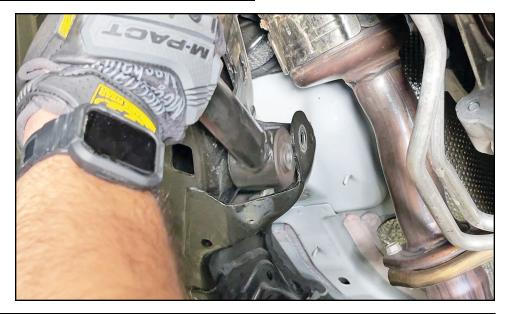
Insert the tops of the new brackets in to the factory upper control arm frame brackets and insert the factory upper control arm frame bolts thru them as shown.
