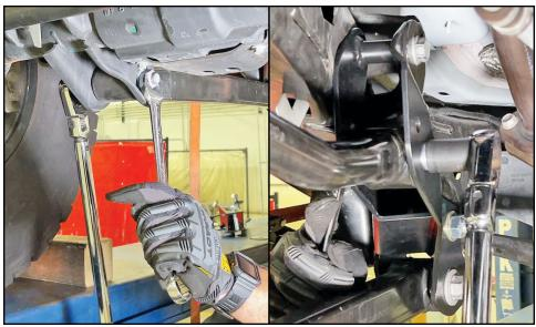
Step 18 Torque all 4 control arm bolts to spec. With this, you are done!
