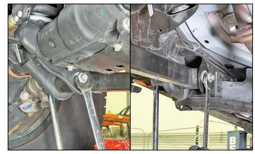
Drop the frame end of the lower control arm out of the bracket and let it swing down out of the
