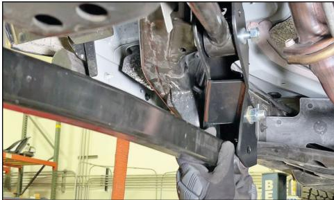
Step 15 Swing the frame ends of the lower control arms up and into the new brackets.
