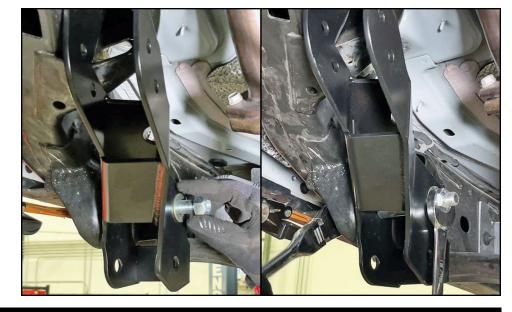
Install the front upper control arms back onto the front axle housing and into the new frame brackets.
